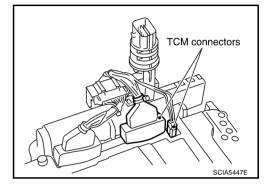
d. Install O-ring to A/T assembly harness connector.
