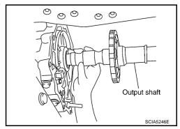
11. Remove parking gear from output shaft.
