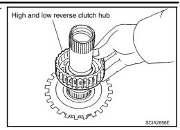
a. Remove needle bearing from high and low reverse clutch hub.
