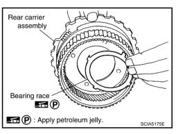
21. Remove needle bearing from rear carrier assembly.
