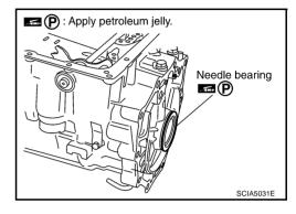
24. Install revolution sensor to transmission case.
