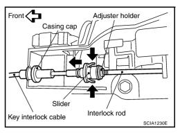
Remove holder from key cylinder and remove key interlock cable
