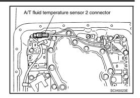
12. Straighten terminal clips to free terminal cord assembly and A/T fluid temperature sensor 2 harness.
