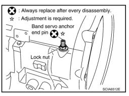
49. Install brake band in transmission case.
