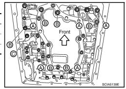
16. Remove control valve with TCM from transmission case.
