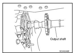
9. Install bearing race to output shaft.
