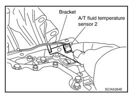
6. Install A/T fluid temperature sensor 2 (with bracket) in control valve with TCM.
