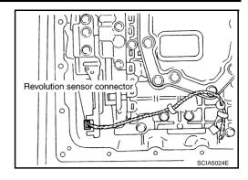
34. Straighten terminal clips to free revolution sensor harness.
