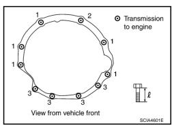
Align the positions of tightening bolts for drive plate with those of the torque converter, and temporarily tighten the bolts. Then, tighten the bolts with the specified torque.
