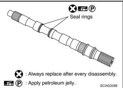
7. Install parking gear to output shaft
