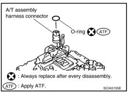
e. Install A/T fluid temperature sensor 2 to bracket.
