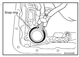
68. Remove servo assembly (with return spring) from transmission case.
