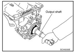
33. Install bearing race to output shaft.
