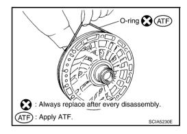
2. Install O-ring to oil pump housing.
