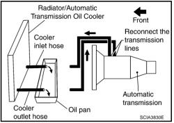
Insert the extension adapter hose of a can of the Transmission Cooler Cleaner (Nissan P/N 999MP-AM006) into the cooler outlet hose.
