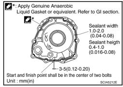
11. Install rear extension assembly to transmission case. (With needle bearing.)
