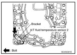
7. Install control valve with TCM in transmission case.
