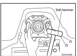
12. Remove rear extension assembly from transmission case. (With needle bearing.)
