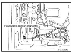
14. Straighten terminal clips to free revolution sensor harness.
