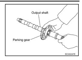
12. Remove seal rings from output shaft.
