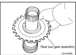
a. Using a flat-bladed screwdriver, remove snap ring from rear sun gear.
