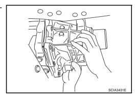
12. Tighten rear extension assembly mounting bolts to specified torque.
