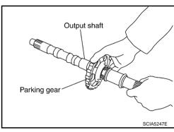
8. Install output shaft to transmission case.
