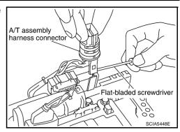
22. Disconnect TCM connector and park/neutral position switch connector.
