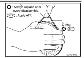
4. Remove O-ring from oil pump cover.
