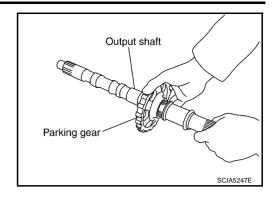
32. Install output shaft in transmission case.
