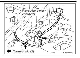
15. Remove revolution sensor from transmission case.
