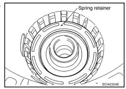
56. Remove seal rings from drum support.
