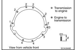
Align the positions of tightening bolts for drive plate with those of the torque converter, and temporarily tighten the bolts. Then, tighten the bolts with the specified torque.
