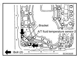
10. Remove bracket from A/T fluid temperature sensor 2.
