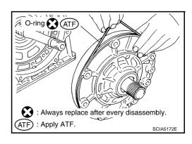
Remove bearing race from oil pump assembly.
