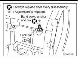
15. Remove brake band from transmission case.
