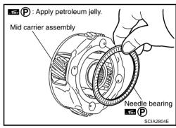
44. Install needle bearing (front side) to mid carrier assembly.
