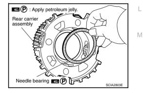
41. Install bearing race in rear carrier assembly.
