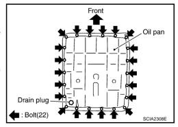
Tighten oil pan mounting bolts to the specified torque in numerical order as shown in the figure after temporarily tightening them.
