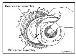
18. Remove needle bearing (front side) from mid carrier assembly.
