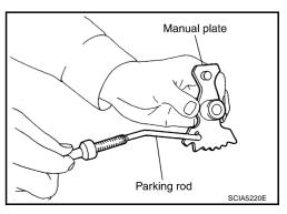
64. Remove manual shaft from transmission case.
