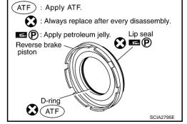
13. Install reverse brake piston in transmission case.
