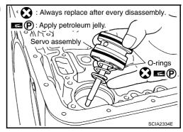
69. Remove return spring from servo assembly.
