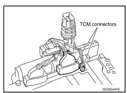
21. Remove A/T assembly harness connector from control valve with TCM using a flat-bladed screwdriver.
