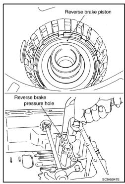
59. Remove lip seal and D-ring from reverse brake piston.
