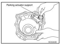
72. Remove parking pawl (with return spring) and pawl shaft from rear extension (2WD models) or adapter case (AWD models).
