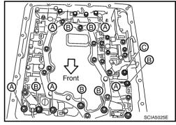
i. Tighten bolt 1, 2 and 3 temporarily to prevent dislocation. After that tighten them in order (1  $\rightarrow$  2  $\rightarrow$  3), and then tighten other bolts.
