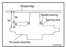
a. Place bearing race and needle bearing on oil pump assembly.
