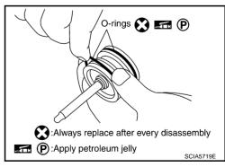
Install return spring to servo assembly.
