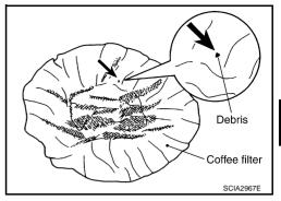
b. If one or more pieces of debris are found that are over 1mm (0.040 in) in size and/or peeled clutch facing material is found in the coffee filter, the fluid cooler is not serviceable. The A/T fluid cooler/radiator must be replaced and the inspection procedure is ended.Refer to CO-14, "RADIATOR" and CO-17, "RADIATOR (ALUMINUM TYPE)" (for VQ35DE), CO-39, "RADIATOR" and CO-43, "RADIATOR (ALUMINUM TYPE)" (for VK45DE).
