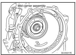
17. Remove mid carrier assembly from rear carrier assembly.
