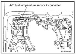
32. Straighten terminal clips to free terminal cord assembly and A/T fluid temperature sensor 2 harness.
