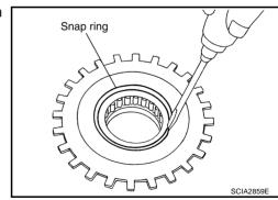
o. Remove 1st one-way clutch from rear sun gear.
