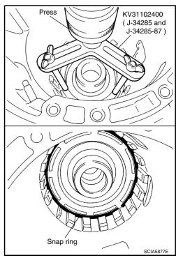
18. Install reverse brake drive plates, driven plates and dish plate in transmission case.
