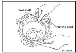
4. Install parking actuator support to rear extension.
