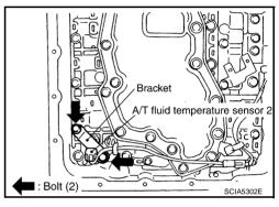
3. Connect A/T fluid temperature sensor 2 connector.
