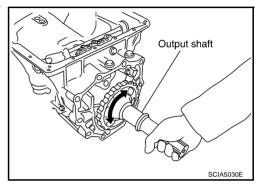
46. Remove parking gear from output shaft.
