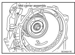
46. Install front carrier assembly, input clutch assembly and rear internal gear as a unit.
