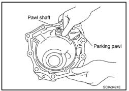
28. Install parking actuator support to rear extension (2WD models) or adapter case (AWD models).
