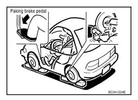
6. Start the engine, then measure the line pressure at both idle and the stall speed.
