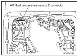
4. Securely fasten A/T fluid temperature sensor 2 harness with terminal clip.
