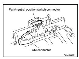
Install A/T assembly harness connector from control valve with TCM.
