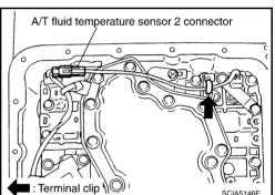
9. Remove A/T fluid temperature sensor 2 with bracket from control valve with TCM.
