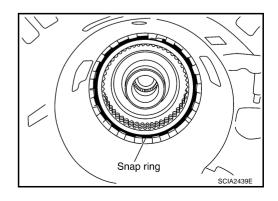
22. Measure clearance between retaining plate and snap ring. If not within specified clearance, select proper retaining plate.
