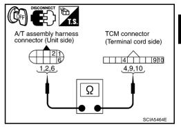
Check continuity between A/T assembly harness connector terminals and TCM connector terminals.
