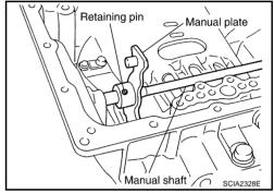
61. Remove manual shaft retaining pin with nippers.
