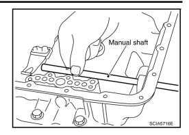
65. Remove manual shaft oil seals using a flat-bladed screwdriver.
