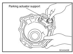
15. Remove parking pawl (with return spring) and pawl shaft from rear extension.
