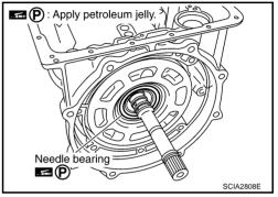
11. Remove front sun gear assembly from front carrier assembly. NOTE:
