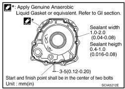
Install rear extension assembly to transmission case. (With needle bearing.)
