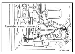
13. Securely fasten revolution sensor 2 harness with terminal clips.
