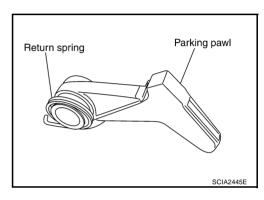
3. Install parking pawl (with return spring) and pawl shaft to rear extension.
