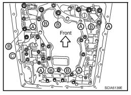
9. Tighten bolt 1, 2 and 3 temporarily to prevent dislocation. After that tighten them in order  $(1 \to 2 \to 3)$ , and then tighten other bolts.
