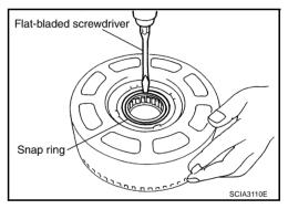
2. Remove 3rd one-way clutch from front sun gear.
