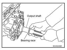
10. Remove output shaft from transmission case by rotating left/ right.
