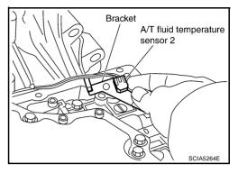
2. Install A/T fluid temperature sensor 2 (with bracket) in control valve with TCM.
