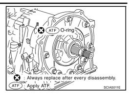
Remove tightening bolts for oil pump assembly and transmission case.
