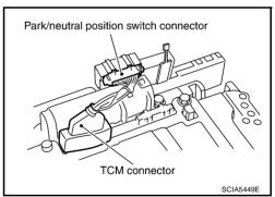
Install A/T assembly harness connector from control valve with TCM.
